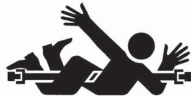
Do not wear loose fitting equipment around rotating drivelines. Stop the engine and make sure that all moving parts have stopped before making any adjustments, connections, or performing any other type of service to the engine or other driven equipment.
