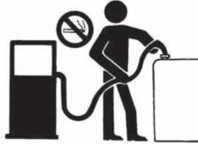
Prevent accidental discharge of starting fluids by storing all cans in a cool, safe place, away from sparks or open flame. Store with cap securely on container. Never incinerate or puncture a fuel container.
