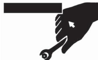
Use power tools only to loosen threaded parts and fasteners. For loosening and tightening hardware, always use the correct sized tools. Do not use US measurement tools on metric fasteners, or vice versa. Use only service parts that meet Northern Lights specifications.
