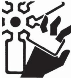
Do not allow anything on your person to dangle into or come in contact with a moving fan, belt, pulley or drive. Fans can act as vacuums and pull materials up from below, so avoid that area as well while in service.
